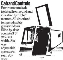
controllers for swing, winches and boom hoist. Foot controls for swing brake and boom telescope.
