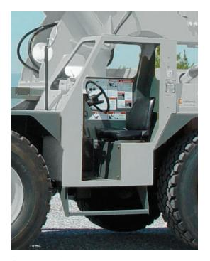
Standard: Open air cab shell w/overhead safety
