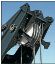
bearings and pin-on lugs for attachment options such as a fixed jib and auxilary tip extension. In-line boom suspension load cell, standard with anti-two block system
