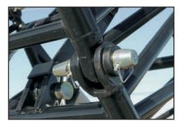
↑ Double tapered connecting pins allow installation/removal from outside of boom. Boom connecting pins store in picture frame of boom extensions for transport.
