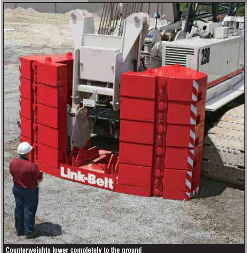
Counterweights lower completely to the ground
