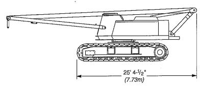
Assembly Weight - as shown 85,250 lbs. (38 669 kg) w/Live Mast and rope on one drum 82,550 lbs. (37 445 kg) w/o Live Mast and rope on one drum
