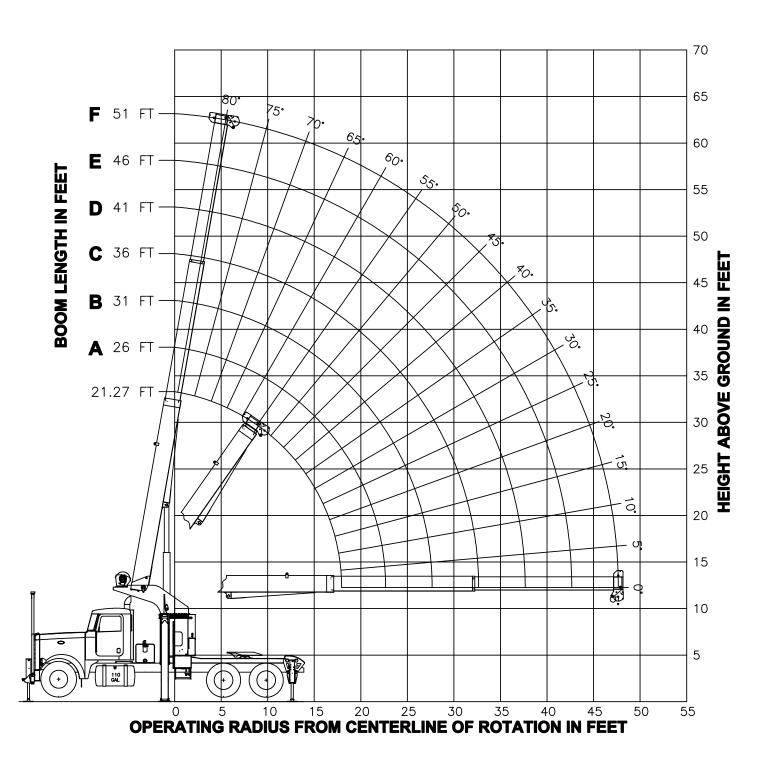
Lifting Capacities 3-section Boom 30 ft. - 100 ft. Jib 26 ft. - 46 ft.
